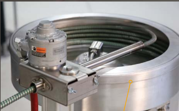
HOSE CONTAINMENT DRUM For safe management and storage of high-pressure hose
