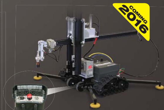
WIRELESS CONTROL & TRACK BASE Reposition Striker and maintain line of sight from outside the blast zone.
