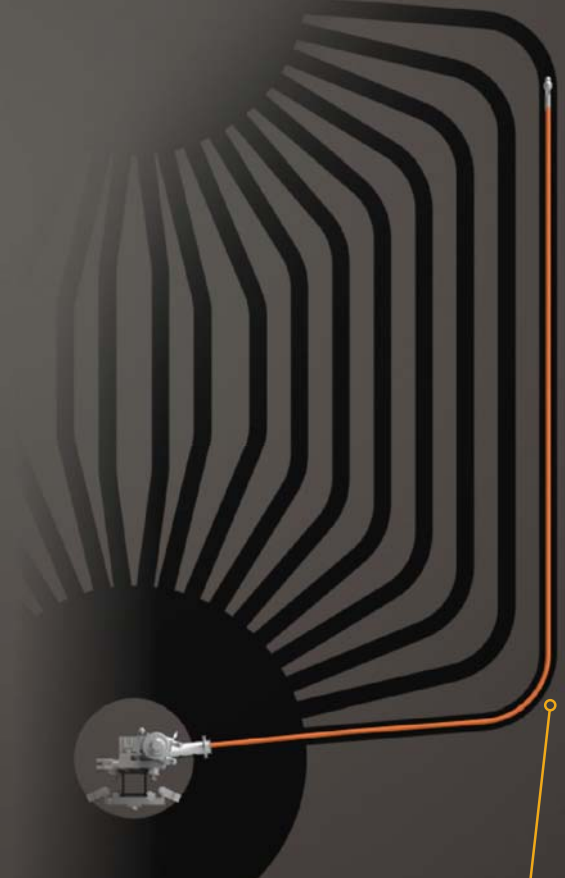
PRECISE, CONTROLLED HOSE FEED Allows cleaning through multiple tube bends while protecting hose from damage
