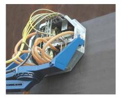
The blasting head seals directly onto the hull surface and is connected to the vacuum unit via a hose/pipework combination
