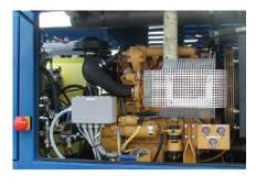
The hydraulic installation comprises two independent circuits each powered by a pump. The system is controlled by proportional valves, solenoid valves, pressure limiting valves combined with hydraulic motors and hydraulic cylinders. The hydraulic pumps are driven by a water cooled CAT diesel engine.
