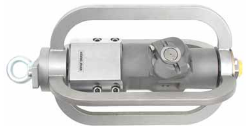
Type XL 1600-2 with sledge for pipe cleaning 35 mm S-arm, 2 nozzles max. 1600 bar / 250 l/min. Min. Pipe -Ø: 320 mm
